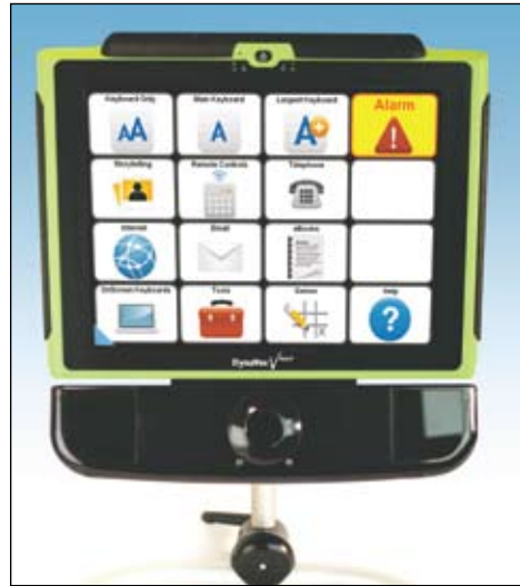
The DynaVox Vmax speech communication device, typically used in a stationary position on a desktop or wheelchair mount, and the DynaVox EyeMax, a new and advanced eyegaze system for accessing the device.
