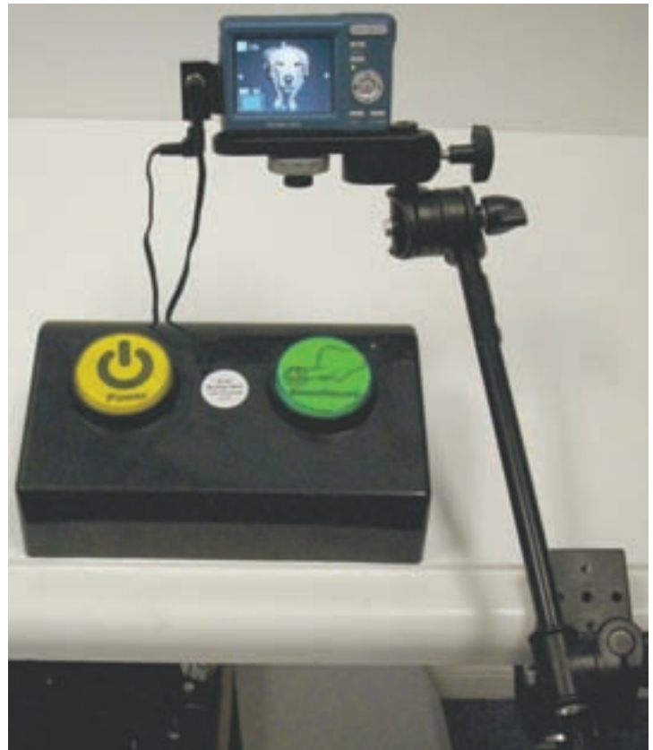
Dual Button box shown plugged into my Switch-Adapted Digital Camera.
