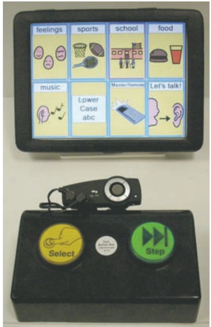
Dual Button box shown plugged into my cordless Super-Switch, operating my AAC software, PTP-PC, on my Super-Auggie AAC device, with step-scan labels in buttons
