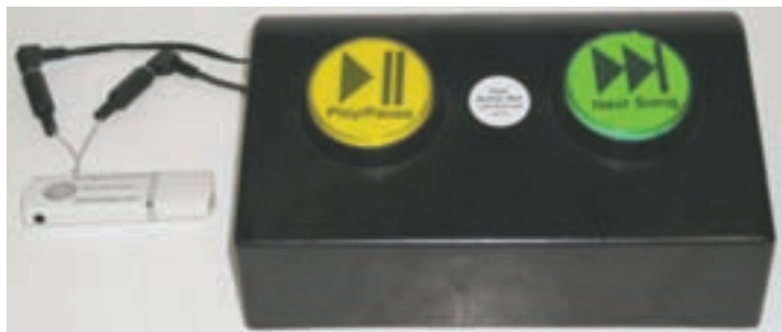
The Dual Button Box shown with Switch-Adapted MP3 Player/Drive on left, and associated labels in the buttons.
