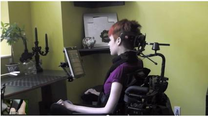
Tecla brings smart device access to all. It connects people with limited physical mobility to technology. Tecla allows interaction with iOS and Android devices via the specialty switches or wheelchair driving controls that are already used.
