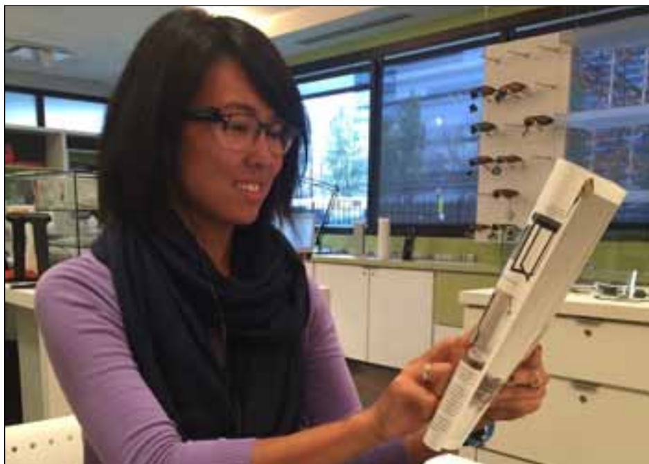
Using the OrCam it is possible to simply point at the text you wish to have read. The OrCam's camera, mounted on the user's glasses, detects where the user's finger is pointing and reads the text through a speaker mounted next to the right ear
