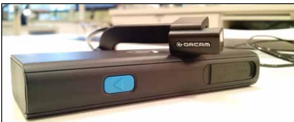
The OrCam is very compact, making it comfortable to wear for long periods. The camera (pictured on top) fits onto the user's eyeglasses and is connected to the computer (pictured at bottom) by a wire.
