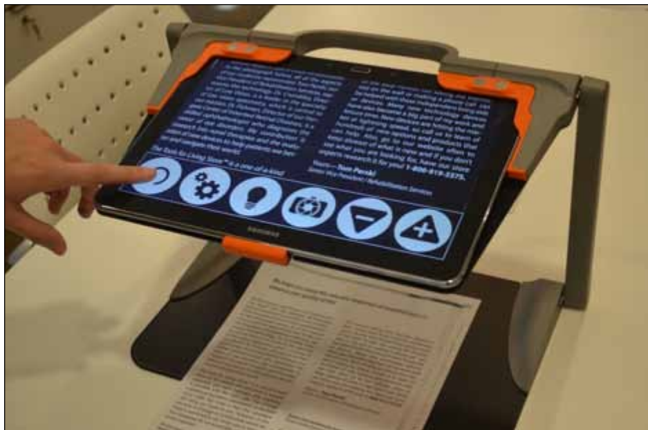
The Prodigy Connect 12 from Humanware is a good example of the convergence of different areas of assistive technology, featuring distance and near viewing, OCR/TTS and access to all Android features and apps in the Google Play store.
