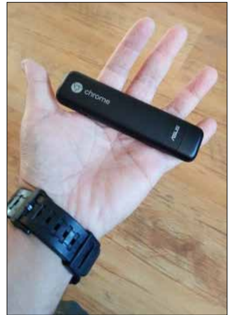
Image 1: Chromebit is a Chrome computer on a USB-style drive that will change any HDMI display into a computer.
