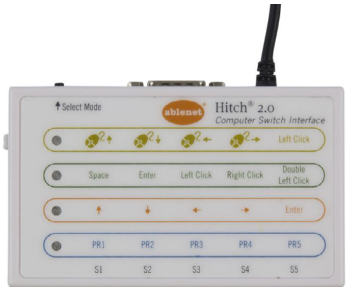
Image 2: Hitch 2 is a USB switch interface available by AbleNet, Inc.
