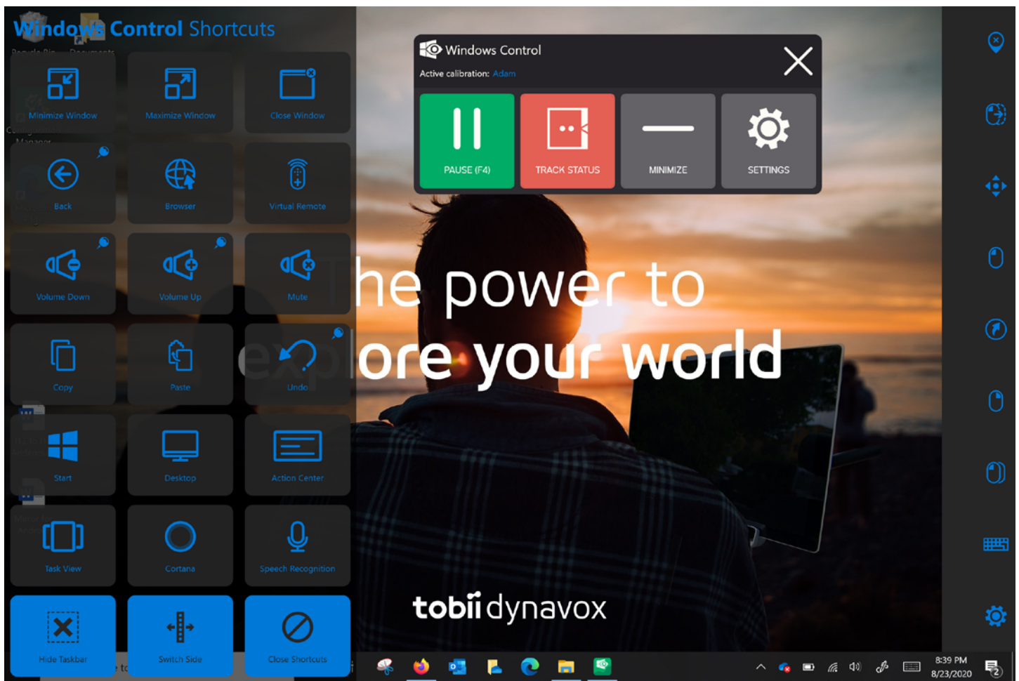
Image 5: A pop-up of the 21 different Windows Control shortcuts that appears on the left side of the screen.
