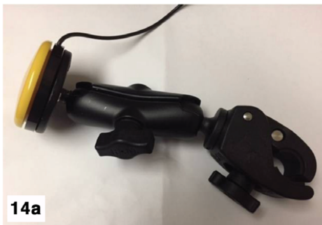
Image 14a: A Ram Mount (Rammount.com) is used to mount a switch to a child's walker.
