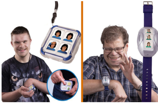
A watch-sized, nine message, wearable AAC device
