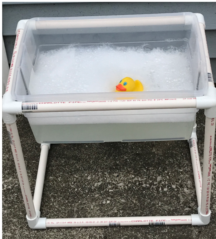
Image 7: Height sensory table constructed from PVC pipe, connectors, and a plastic tub with lid can be filled with a variety of items. Table can be disassembled and stored in tub.
