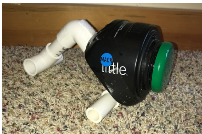
Image 12: PVC switch holder allows the user to use a swipe motion to contact switch.
