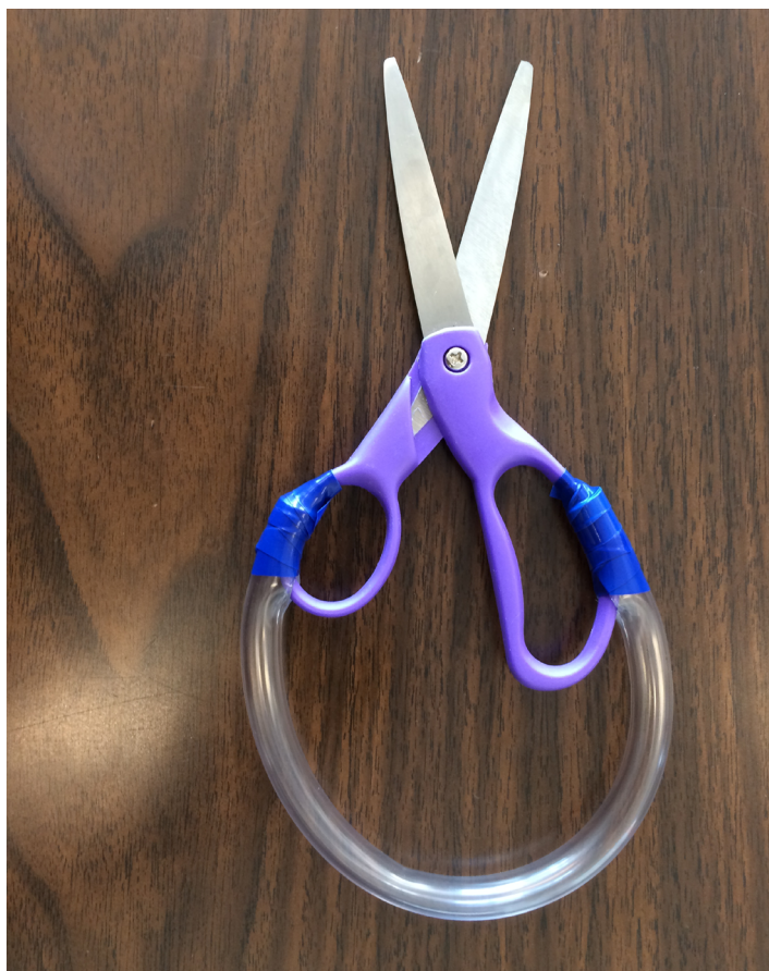
Figure 4: Improvised spring-loaded scissors using aquarium tubing secured with duct tape
