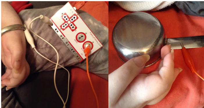
An example of the Makey Makey board connected to a computer with the ground wire clipped to a metal bracelet and the input wire clipped to a metal measuring cup. The circuit is activated once the user lightly touches the cup.
