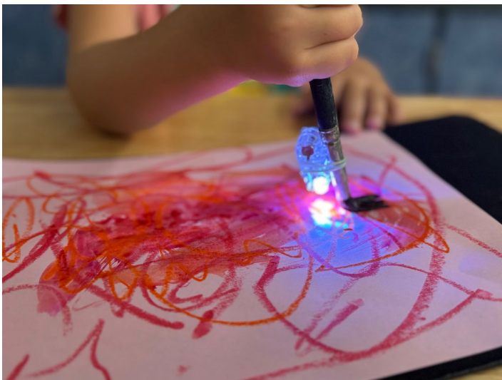
A fingerlight attached to a paintbrush handle illuminates the surface as the user watercolors, with the caption "DIY adaptive light-up paintbrush supporting creative expression."
