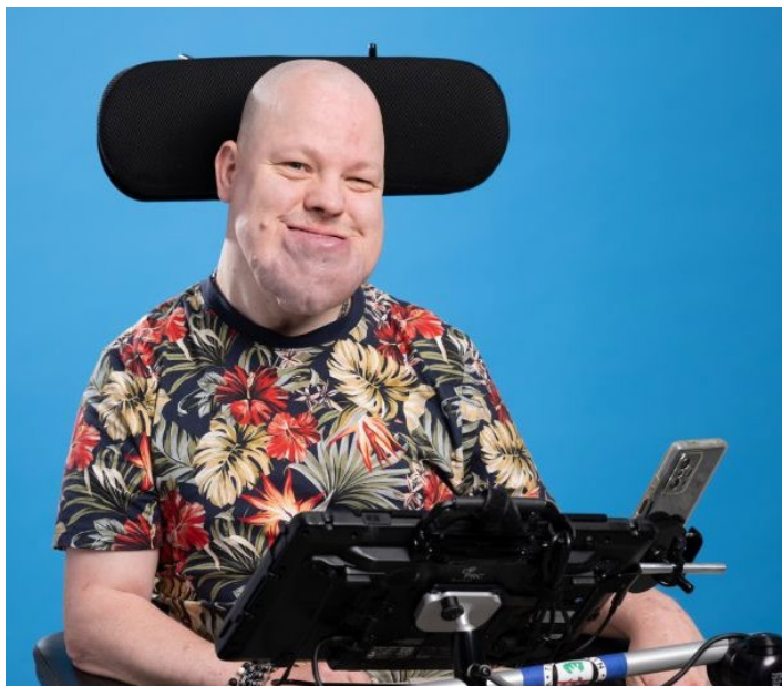
Frank with his SGD mounted on a wheelchair with a M3D mount with a swing away joint. His phone is attached directly to the Accent 1400 using a dedicated phone holder.
